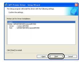
If you are using an operating system equipped with Windows Firewall, such as Windows XP Service Pack 2, the following window is displayed. Click [No].
